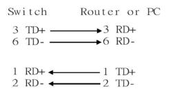
Straight Through Cable Schematic
